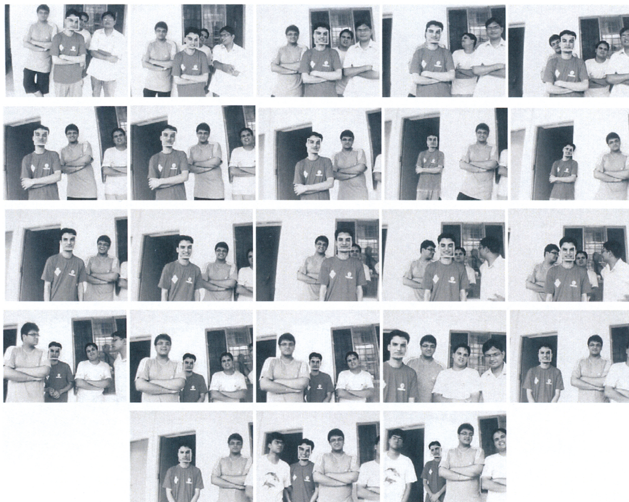
Fig. 6. Video sequence showing the face tracking of desired subject under various complex motion, introduction of new human subject and partial occlusion. Note that the subject was chosen in first frame by the proposed heuristic of searching for the most prominent face and tracked throughout the rest of the video.
